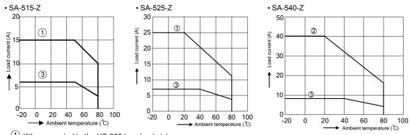
• (1) When mounted to the HS-320 type heat sink.
